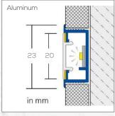
For floor insertion, seal with **DURALIS-LED** adhesive tape DLK
